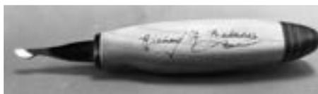
**Richard Belcher Signature Knife** made by Helvie Knives. Blade is a 3/8" curved broadax shape. Excellent tool for cleanup in tight places. Allows for pushing cuts. **Sharpened.**
